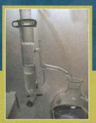
Unlike other steam distillation units on the market, EVS2000 offers true *dry steam* distillation in an all glass (Pyrex) system. Coupled together with ground glass joints, there are no hoses or rubber stoppers in contact with your product ... it's all glass!
